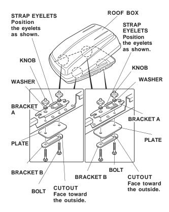
5. Fit bracket A over the threads of the bolt where it protrudes through the roof box. Install a washer over the threads, and loosely install a knob. Install a second bolt the same way. Install bracket A with the right and left strap eyelets directly across from each other. 6. With the help of an assistant, carefully place the box on the crossbars. Be careful not to damage the crossbars or the roof with the hardware hanging from the bottom of the box.
