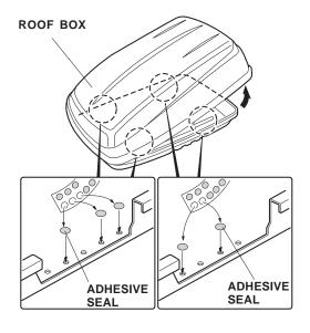
2. Using isopropyl alcohol on a shop towel, clean four brackets B where the small pads will attach. Remove the adhesive backings from the small pads and attach them to the brackets B.
